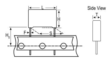
Series R75 Dielectric Metallized Polypropylene Style Radial Features Automotive Grade, Pulse RoHS Lead Wire Leads Qualifications AEC-Q200 AEC-Q200 Yes Component 4.87 g Weight Above 85C DC And AC Voltage Derating Is Miscellaneous 1.25%/C.
