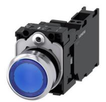
Illuminated pushbutton, 22 mm, round, Metal, shiny, blue, pushbutton, flat, momentary contact type, with holder, 1 NO+1 NC, LED module with integrated LED 230 V AC, spring-type terminal, with laser labeling, inscription or symbol Customer-specific selection with SIRIUS ACT configurator (CIN)
