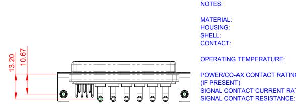
THERMOPLASTIC POLYESTER, UL94V-0 STEEL, TIN PLATED COPPER ALLOY, GOLD FLASH PLATED
