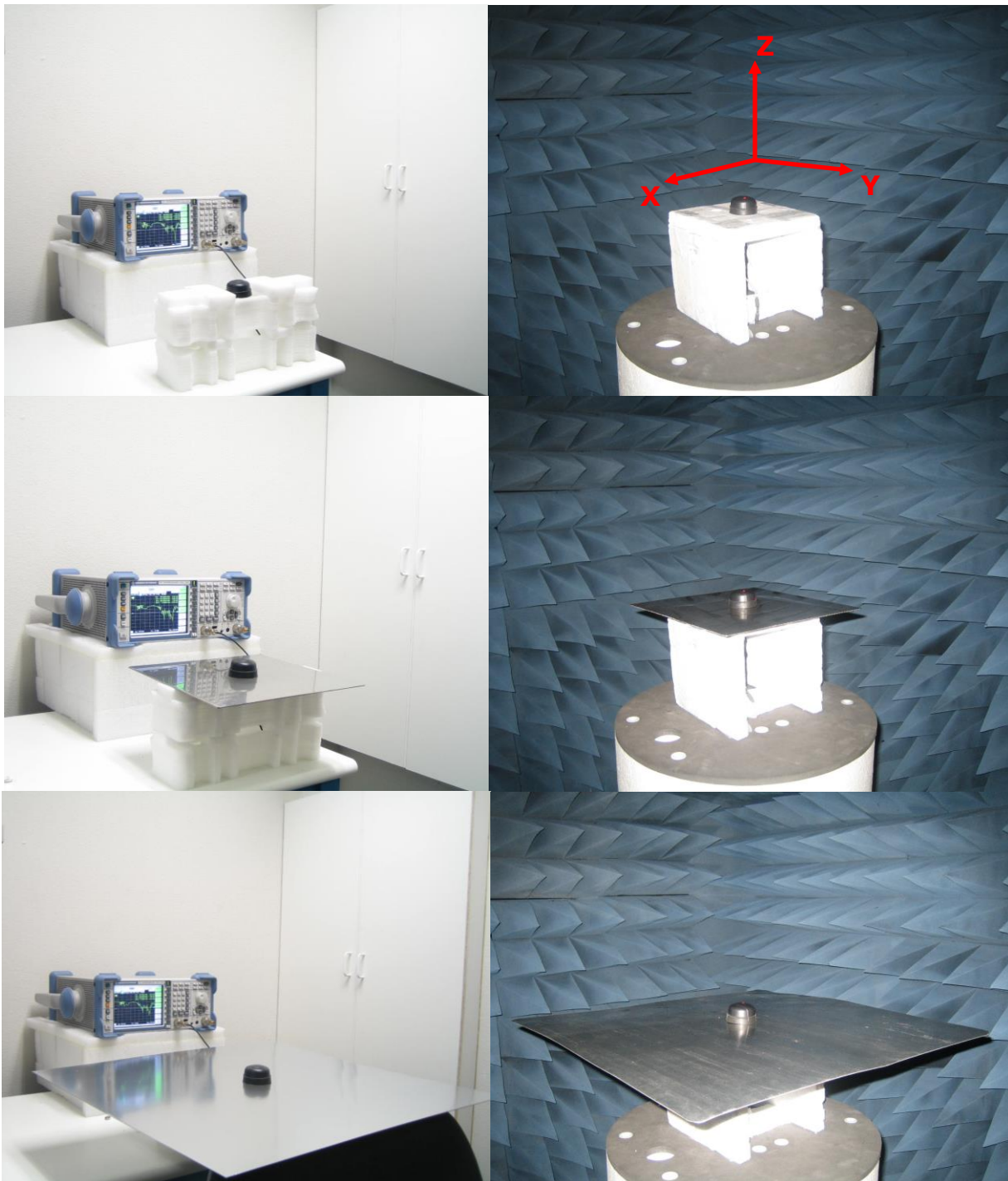
Figure 1. IS.05 Antenna test set up in free space, 30x30cm metal plate and 60x60 cm metal plate, R&SZVL6 VNA (left) and R&S4100 CTIA 3D Chamber (Right).
