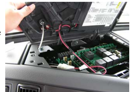
Tilting and Removal of Top
