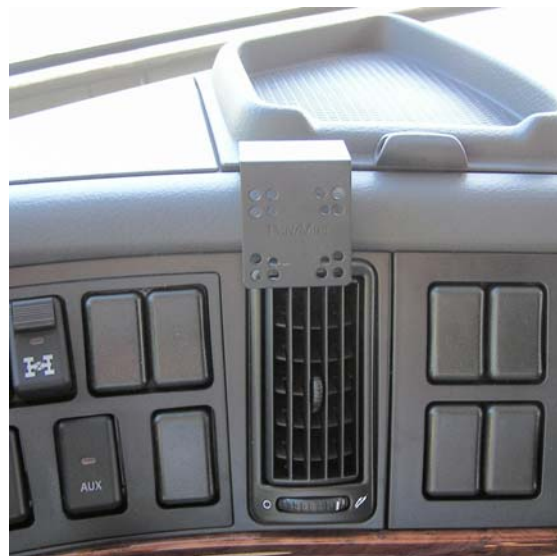
InDash installed showing South direction with 75006 part
