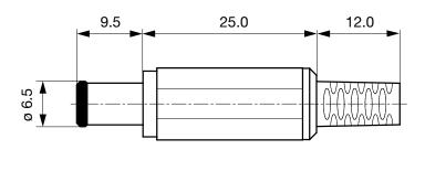
Cable diameter max. 4.0 mm
