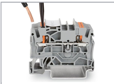
Insert fine-stranded conductors via operating tool.
