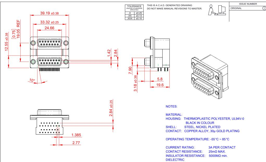
WITHSTANDING VOLTAGE: 1000V AC rms
