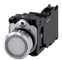
Illuminated pushbutton, 22 mm, round, Metal, shiny, transparent, pushbutton, flat, momentary contact type, with holder, 1 NO+1 NC, LED module with integrated LED 230 V AC, spring-type terminal, with laser labeling, upper case and lower case, always upper case at beginning of line
