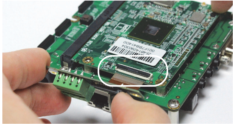
Figure 31: Connecting adapter board and embedded board
