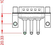
20A (CURRENT) POWER/CO-AX CONTACT RATING: (IF PRESENT) SIGNAL CONTACT CURRENT RATING: 5A PER CONTACT SIGNAL CONTACT RESISTANCE:  $10m\Omega$  MAX.
