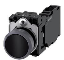
Pushbutton, 22 mm, round, plastic with metal front ring, black, pushbutton, flat, momentary contact type, with holder, 1 NO+1 NC, screw terminal, with laser labeling, lower case
