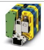
Installation ground terminal block, PE/N block, consisting of a green-yellow ground terminal and a blue terminal block with screw bridge, Screw connection, cross section: 16 mm<sup>2</sup> - 50 mm<sup>2</sup>, AWG: 6 - 1/0, width: 40 mm, color: green-yellow, mounting type: NS 35/7,5, NS 35/15, NS 32
