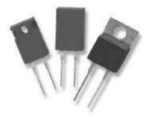
The MPT Resistor series are a range of T0220 and TO247 packaged, low inductance thick film power resistors. This small size, high power device with 5 models are ideally suited to applications where high power dissipation yet small size are key design requirements. The MPT Resistor series are the ideal solution for small snubber circuits, the output side of high speed pulse generators and low inductive resistor requirements in switch mode power supplies.
