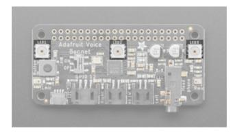
Three fully color RGB addressable LEDs can provide feedback or a light show. Uses DotStar protocol (not NeoPixel) so any microcomputer can easily control the lights.
