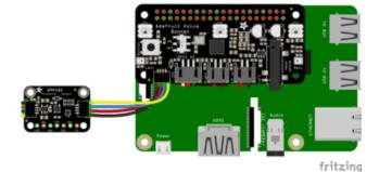
Connect one side of the Stemma QT cable to either port on the BMP280 Connect the other side to the Stemma QT port on the Voice Bonnet
