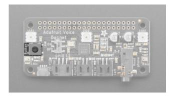
This pin has a 10K pullup to 3.3V so when the button is pressed, you will read a LOW voltage on this pin.
