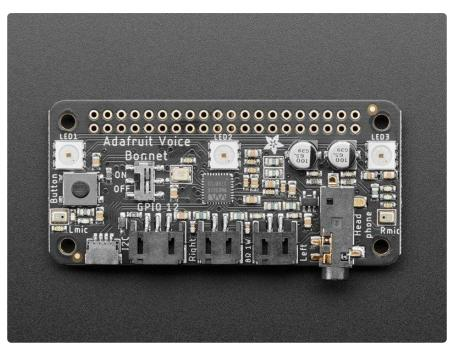
Your Raspberry Pi computer is like an electronic brain - and with the Adafruit Voice Bonnet you can give it a mouth and ears as well! Featuring two microphones and two 1 Watt speaker outputs using a high quality I2S codec, this Pi add-on will work with an y Raspberry Pi with a 2x20 connector - from the Pi Zero up to the Pi 4 and beyond (basically all but the very first ones made).
