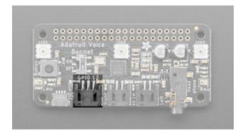
GPIO 12 is accessible with the JST connector on the bottom edge of the Voice Bonnet.
