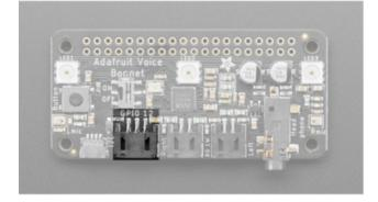
GPIO#12 - 3-pin JST digital or analog connector. Easily connect things like NeoPixels () or servos () using this 2mm connector. You can also use a generic JST cable to connect to a breadboard. ()
