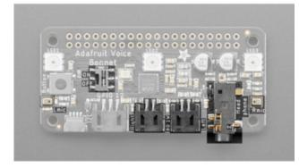
GPIO #18, GPIO #19, GPIO #20, GPIO #21 -I2S Digital Audio.
