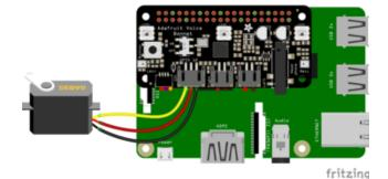
Connect the JST PH 3-pin plug into the GPIO #12 on the Voice Bonnet
