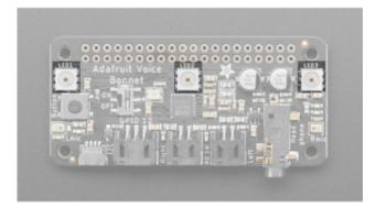
The 3 DotStar LEDS can be controlled with the DotStar CircuitPython Library. Here's a little script that will setup the DotStar LEDs and then color cycle them.
