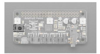
The button uses simple digitalio, so it's really simple to control. Here's a little script that will setup the GPIO, create an internal pull up, and then print out the value to the terminal.
