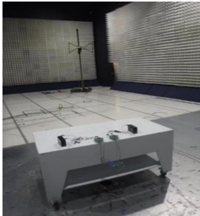
Figure 8. EMI Testing Setup in Chamber
