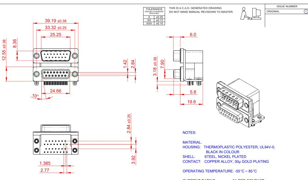
**CURRENT RATING: 3A PER CONTACT** CONTACT RESISTANCE:  $25m\Omega$  MAX. INSULATOR RESISTANCE: 5000MΩ min. DIELECTRIC WITHSTANDING VOLTAGE: 1000V AC rms
