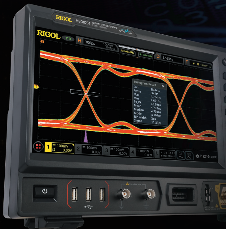
Perform eye measurement on the 622 Mb/s signal.
