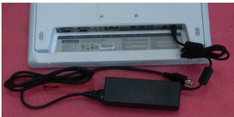
Figure 2.3 Connecting the Power Cord to the DC Inlet
