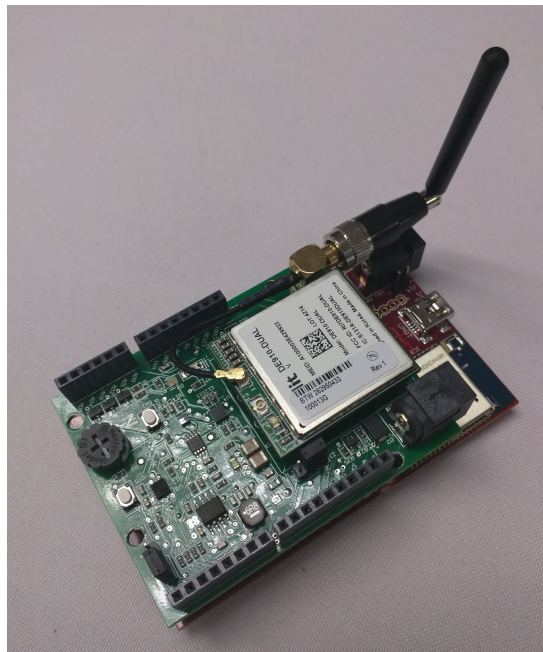
Figure 3-4: Skywire Sensor Shield with Skywire 3G EVDO Modem
