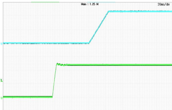
Figure 6: Turn-on transient at zero load current (20 ms/div). Top Trace: Vout; 5V/div; Bottom Trace: input voltage: 30V/div.
