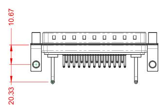
POWER/CO-AX CONTACT RATING:10A (CURRENT)(IF PRESENT)SIGNAL CONTACT CURRENT RATING:5A PER CONTACTSIGNAL CONTACT RESISTANCE:10mΩ MAX.INSULATOR RESISTANCE:5000MΩ min.DIELECTRIC5000MΩ min.
