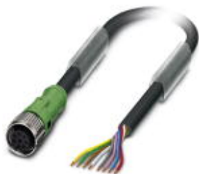
Sensor/actuator cable, 8-position, PUR halogen-free, black-gray RAL 7021, free cable end, on Socket straight M12 SPEEDCON, A-coded, cable length: 3 m
