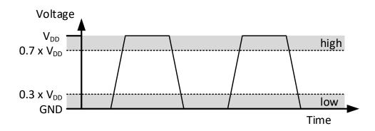
Figure 4: SDA and SCL logic levels
