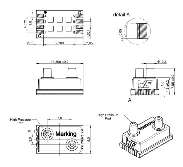
Figure 10: Sensor dimensions [mm]
