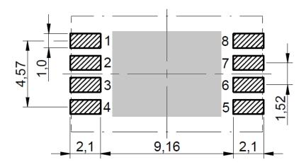
Figure 11: Recommended land pattern [mm] (top view)
