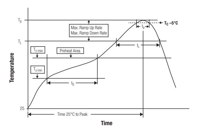
Figure 13: Reflow soldering profile
