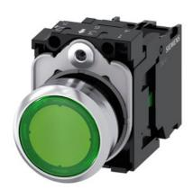
Illuminated pushbutton, 22 mm, round, metal, shiny, green, pushbutton, flat, momentary contact type, with holder, 1NO, LED module with integrated LED 24 V AC/DC, screw terminal, with laser labeling, upper case
