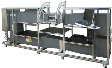
Fig F: FDK Original Wind Tunnel
