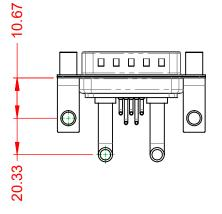
40A (CURRENT) POWER/CO-AX CONTACT RATING: (IF PRESENT) SIGNAL CONTACT CURRENT RATING: 5A PER CONTACT SIGNAL CONTACT RESISTANCE:  $10m\Omega$  MAX.
