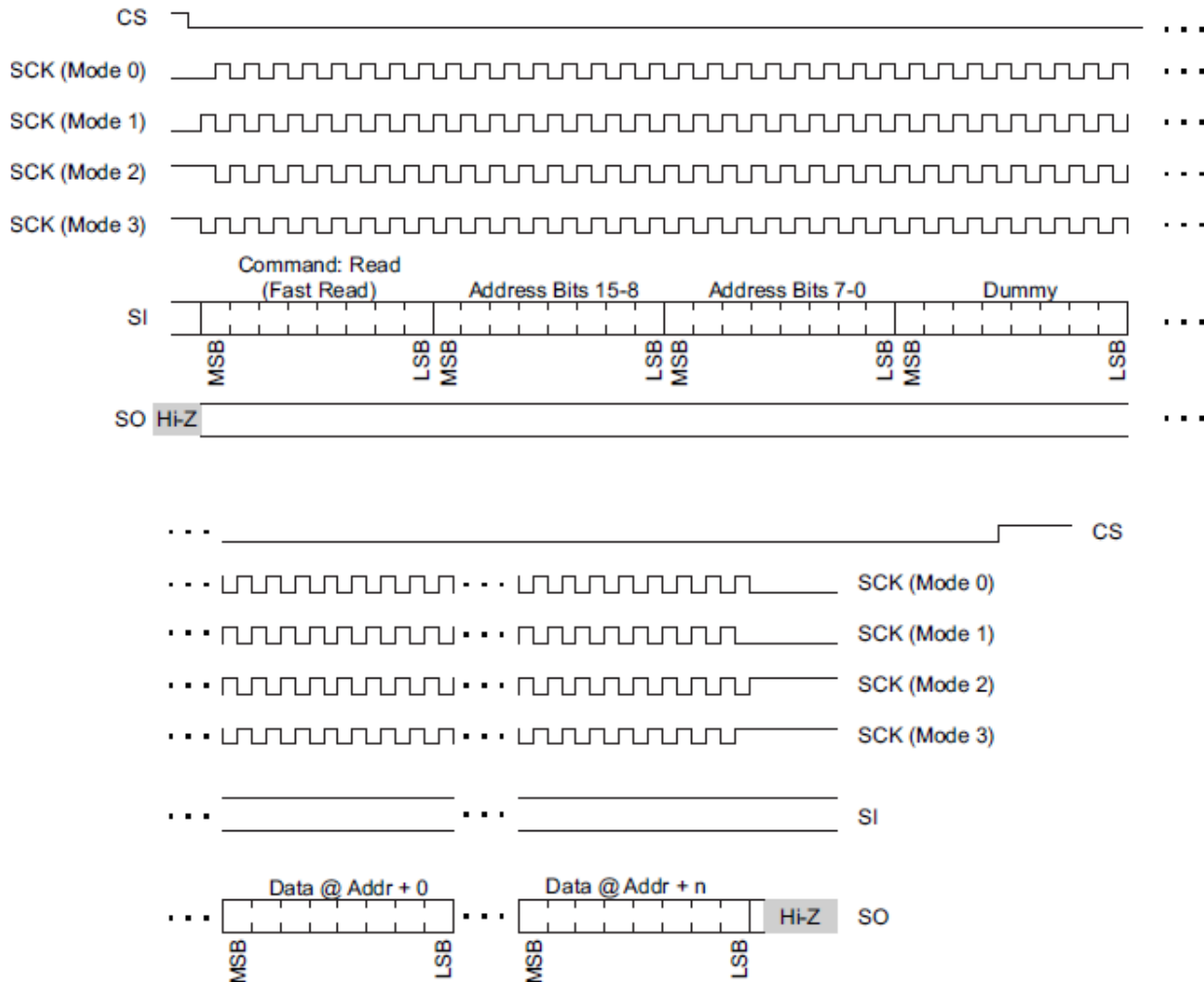
Figure 5. SPI Read Access
