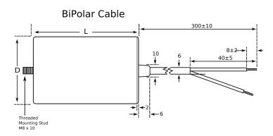
General Information Series C27 Dielectric Film/Foil Polypropylene Style Plastic Case and Cover, Ultra Sonically Welded Description Ultra Sonically Welded Seal, Safety Class PO, **Features** UL 94 V0 Disk RoHS Yes Termination Tin Copper Lead BiPolar Cables UL, VDE, UL (Construction Only), UL\_94 VO Disk Qualifications AEC-Q200 Component 84.93 g Weight
