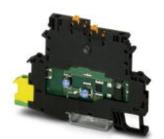
Double-level modular terminal block with two-stage surge protection for one two-wire impedance-sensitive signal circuit, disconnect knife on both signal paths, separate ground connection, nominal voltage: 24 V DC.
