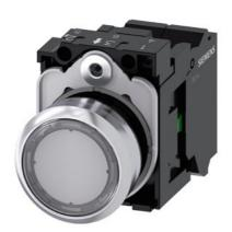
Illuminated pushbutton, 22 mm, round, metal, shiny, clear, pushbutton, flat, momentary contact type, with holder, 1NO, LED module with integrated LED 24 V AC/DC, spring-type terminal, with laser labeling, symbol number according to, ISO 7000 or IEC 60417
