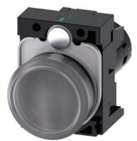
Indicator light with LED lamp, compact, 22 mm, round, plastic, clear with red-yellow-green LED, lens, smooth, with holder, operating voltage 6-24 V AC/DC, screw terminal, with laser labeling, inscription or symbol Customer-specific selection with SIRIUS ACT configurator (CIN)
