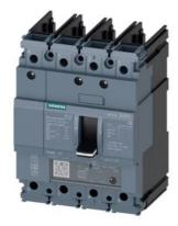
circuit breaker 3VA5 UL frame 125 breaking capacity class S 25kA @ 480V 4-pole, line protection TM230, FTAM, In=125A overload protection Ir=125A fixed short-circuit protection li=5...10 x In N conductor protection 100% without connection
