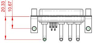
POWER/CO-AX CONTACT RATING: 20A (CURRENT) (IF PRESENT) SIGNAL CONTACT CURRENT RATING: 5A PER CONTACT SIGNAL CONTACT RESISTANCE:  $10m\Omega$  MAX.
