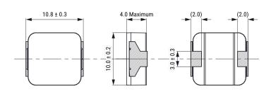
**General Information** Series MPXV Style SMD Chip Size 1040(4340) Description Surface Mount Inductor Features Power Inductors RoHS Yes Qualifications AEC-Q200 AEC-Q200 Yes Core Composite Miscellaneous 40 (K) Temperature Rise Max.
