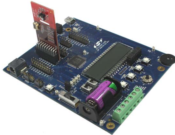
Figure 1. Si7013EVB-UDP Port Header Card Plugged into a UDP SiM3L1xx MCU Card with Multiplexed LCD
