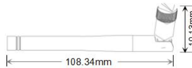
Image 10 | LoRa Antenna Dimension
