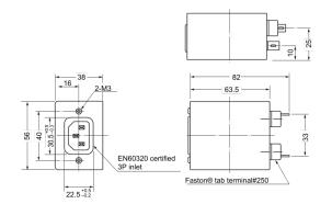
**General Information** Series GL Style Metal Box Description Noise Filters RoHS With Exemptions Qualifications UL, CSA, TUV 30 K Self-Temperature Rise Max. Miscellaneous Lead Screw Terminals **Terminal Type** Screw
