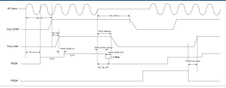
\*NOTE: The PSOK levels after the loss of the incoming AC source may be either 1.1V or 2.2V depending on the relative timing of the TACPOK\_OFF and TPWR\_GOOD\_HOLD-Up
