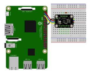
Connect board Vcc (long red wire) to Pi 3.3V
