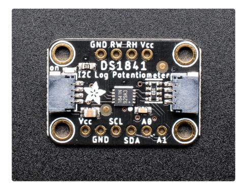
Potentiometers are the perfect tool when you want to change your circuit by turning a knob. Turns out, there are times when you want to adjust your circuit without manually turning a knob, and the DS1841 I2C Logarithmic Resistor from Maxim can do just that. It's a programmable resistor, similar to an I2C potentiometer like the the DS3502 I2C Potentiometer (), so why another?
