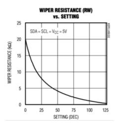
This graph shows the relationship between the wiper setting and the resulting resistance. At the start, the changes are relatively large, but as the values increase, the resulting change in resistance gets smaller and smaller.
