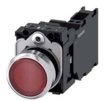
Illuminated pushbutton, 22 mm, round, Metal, shiny, red, pushbutton, flat, momentary contact type, with holder, 1 NO+1 NC, LED module with integrated LED 230 V AC, spring-type terminal, with laser labeling, upper case
