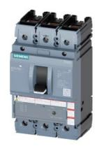
circuit breaker 3VA5 UL frame 250 3-pole, starter protection TM120M, AM, In=200A without overload protection short-circuit protection Ii=3...6 x In cable connection on both sides
