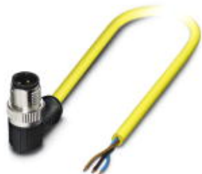
Sensor/actuator cable, 3-position, PVC, yellow, Plug angled M12 SPEEDCON, A-coded, on free cable end, cable length: 10 m
