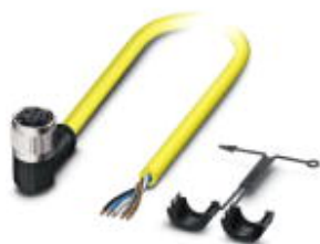
Sensor/actuator cable, 5-position, PVC, yellow, free cable end, on Socket angled M12 SPEEDCON, A-coded, cable length: 5 m
