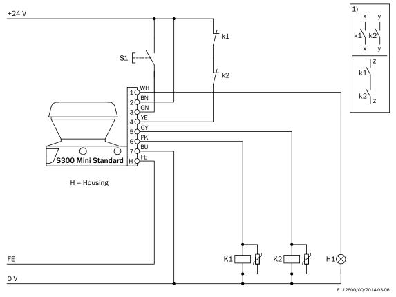
S300 Mini Standard in conjunction with relays/contactors
