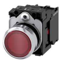
Illuminated pushbutton, 22 mm, round, metal, shiny, red, pushbutton, flat, momentary contact type, with holder, 1NC, LED module with integrated LED 110 V AC, screw terminal, with laser labeling, inscription or symbol Customer-specific selection with SIRIUS ACT configurator (CIN)
