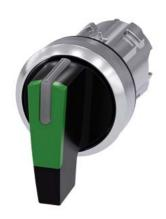
Selector switch, illuminable, 22 mm, round, metal, shiny, green, selector switch, long, 3 switch positions I-O-II, latching, actuating angle 2x45°, 10:30h/12h/13:30h, Z=50-unit packaging
