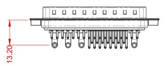
POWER/CO-AX CONTACT RATING: (IF PRESENT) SIGNAL CONTACT CURRENT RATING: 5A PER CONTACT SIGNAL CONTACT RESISTANCE:  $10m\Omega$  MAX. INSULATOR RESISTANCE: 5000MΩ min. DIELECTRIC
