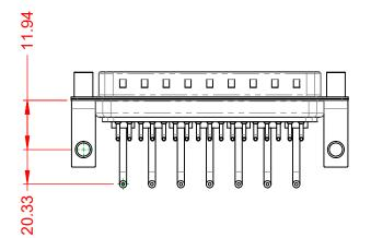
10A (CURRENT) POWER/CO-AX CONTACT RATING: (IF PRESENT) SIGNAL CONTACT CURRENT RATING: 5A PER CONTACT SIGNAL CONTACT RESISTANCE:  $10m\Omega$  MAX. **INSULATOR RESISTANCE:** 5000MΩ min. DIELECTRIC
