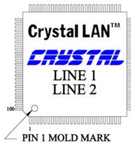
TOP SIDE BRAND Logo Lines (Crystal Lan Logo, Crystal Logo) LINE 1 (PART NUMBER, 14 SPACES MAX) LINE 2 (DATE CODE, 14 SPACES MAX)
